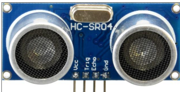
Fig 2: HC-SR04 ultrasonic sensor (Sheldon, 2022)
